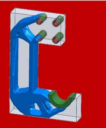
Upon confirmation of the loading through SOLIDWORKS simulation studies, an optimisation was carried out in TruForm SW. The crank set was selected as the designable component with the exception of the pedal, spindle and chain wheel. The load and constraint set defined earlier were selected as the simulation study. The target mass was left at the TruForm default, being 30% of the original design space mass. The outcome was then imported as a graphics body.
