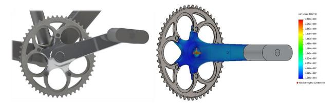
In order to demonstrate the capabilities of TruForm, a typical bicycle crank loading case was selected. The design started as a typical bicycle crank and pedal arm. The chain and axle were represented by constraints. The load applied by a cyclist was represented by a 1000N load at the pedal with example results at one position shown.
