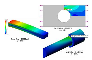
Figure 9: Comparing hand calculations to simulation.
