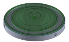
The separate surface and solid bodies in this part are coincident, but also intersect, since the surface is not flat.
