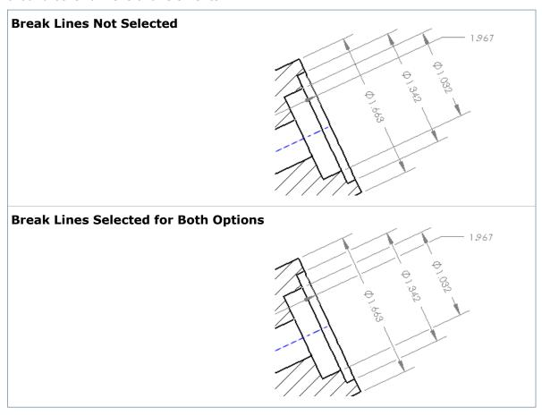
In linear and radial dimensions, you can control which elements of a dimension break around other dimensional elements. On the Leaders tab of the respective PropertyManager, under **Break Lines**:
