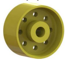
The following image shows the same wheel and appearance, with the **Round Sharp Edges** option enabled and the radius set to 3mm.
